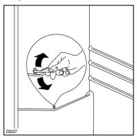
The freezer compartment, however, will become progressively covered with frost. This should be removed with the special plastic scraper provided, whenever the thickness of the frost exceeds 4 mm. During this operation it is not necessary to switch off the power supply or to remove the foodstuffs.
